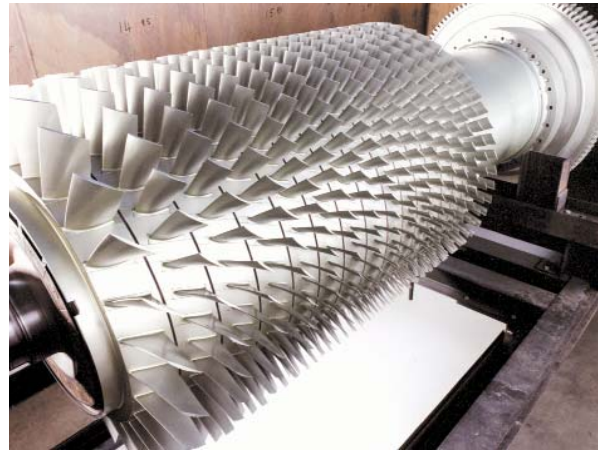
Industrial gas turbine rotor coated with SermeTel 5380 DP.
